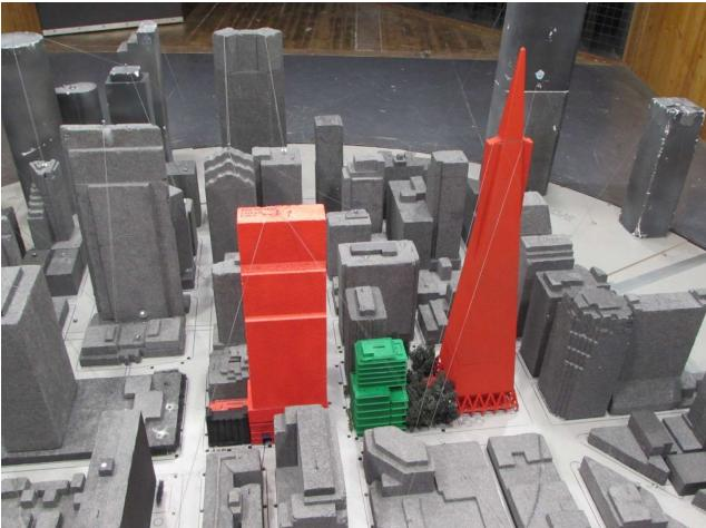
Image 2D: Wind Tunnel Study Model - Project + Cumulative Configuration
