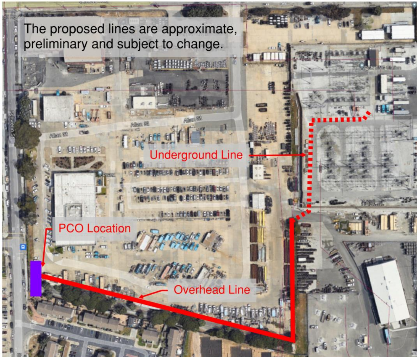
FIGURE 4 Proposed Improvements at the Existing Martin Substation
