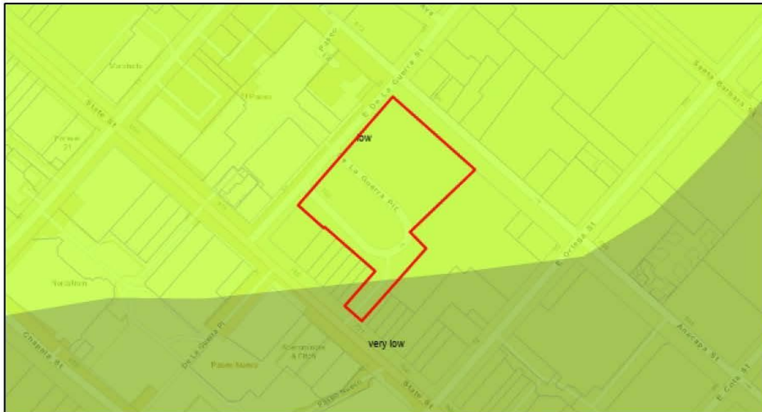
Geological: Landslide Potential
