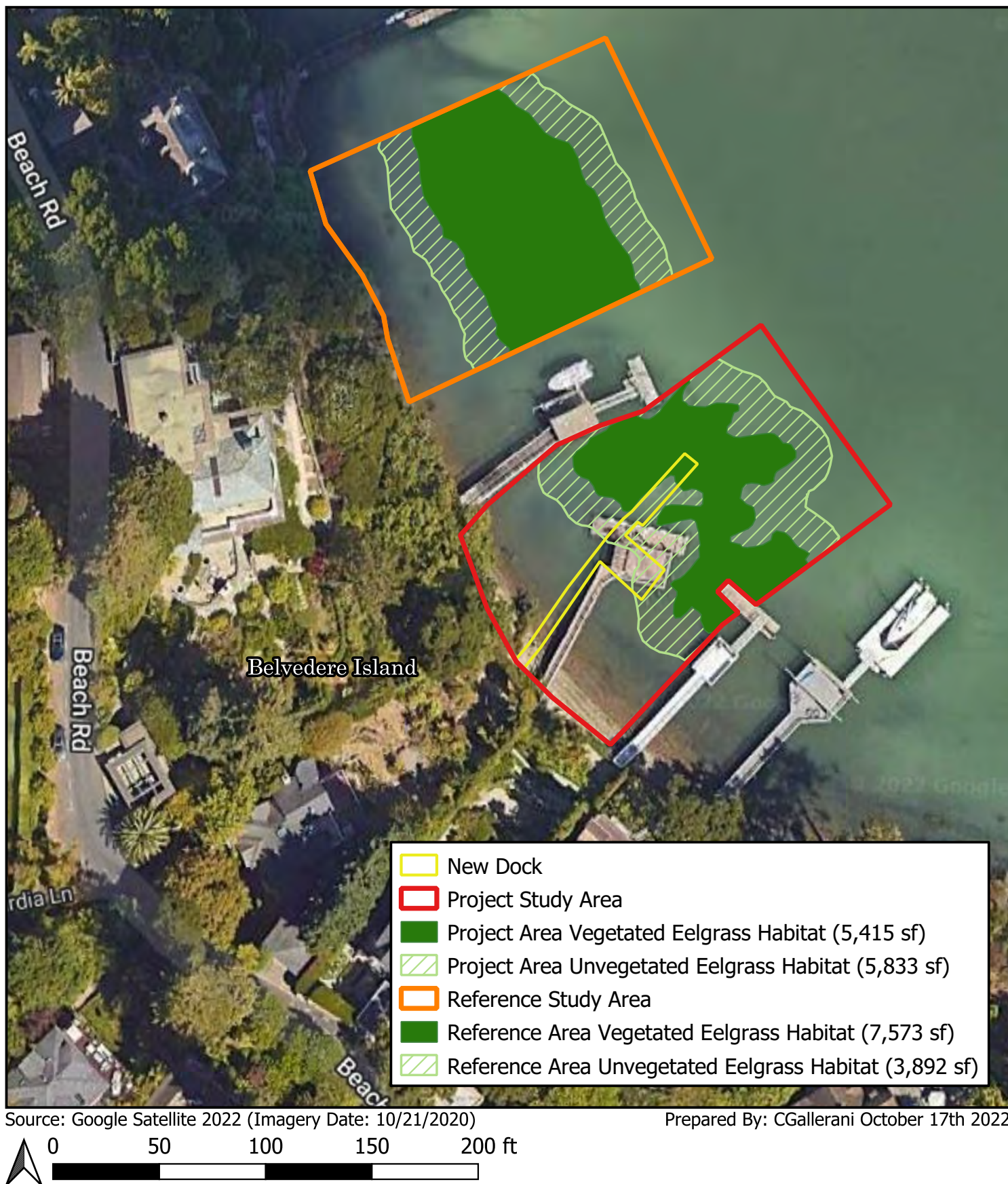
Figure 3. 2021 Post-Construction Eelgrass Survey
