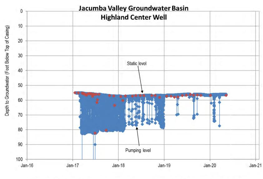
Manual Depth to Groundwater Level Measurement
