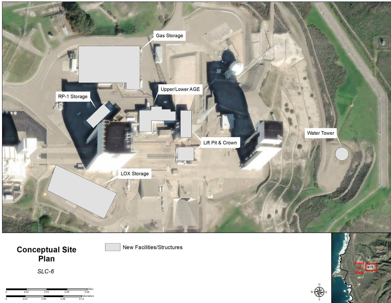
Figure 2.2-2. SLC-6 conceptual site plan; AGE = aerospace ground equipment, LOX = liquid oxygen, RP-1 = rocket propellant-1
