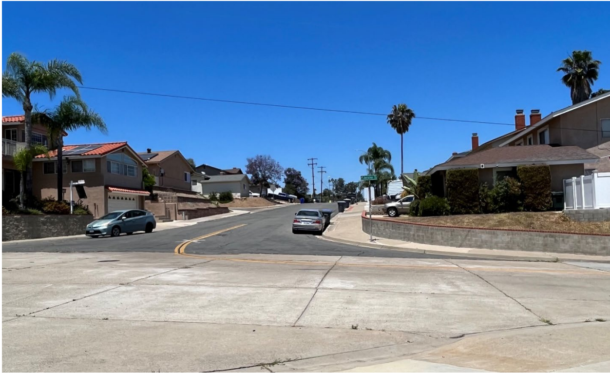
Figure 15 - Corner Sight Distance Looking East from Project Driveway #2 = 466'
