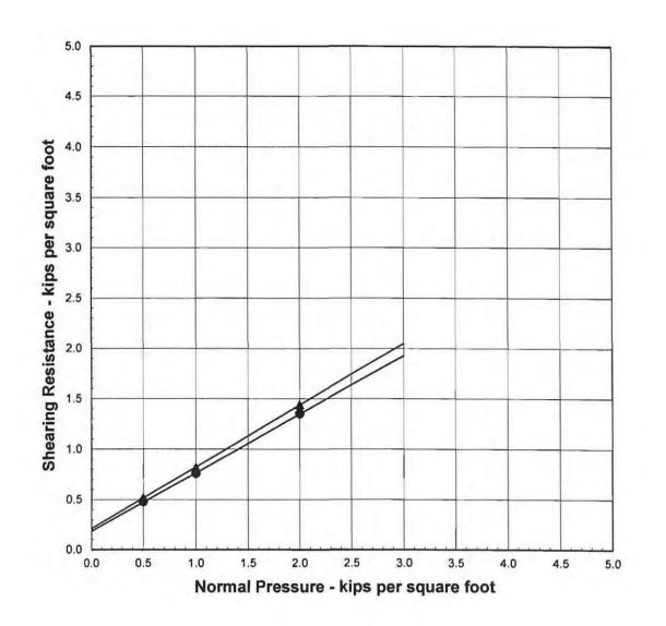
Samples were tested under saturated and drained conditions.
