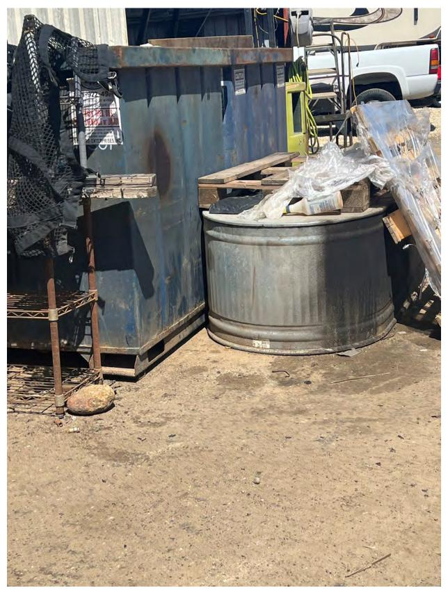
Photo 4: Oil staining on soil, corrosion on metal containers
