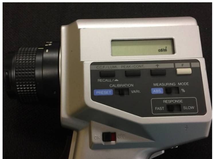
Figure 3: Minolta LS-100 luminance meter
