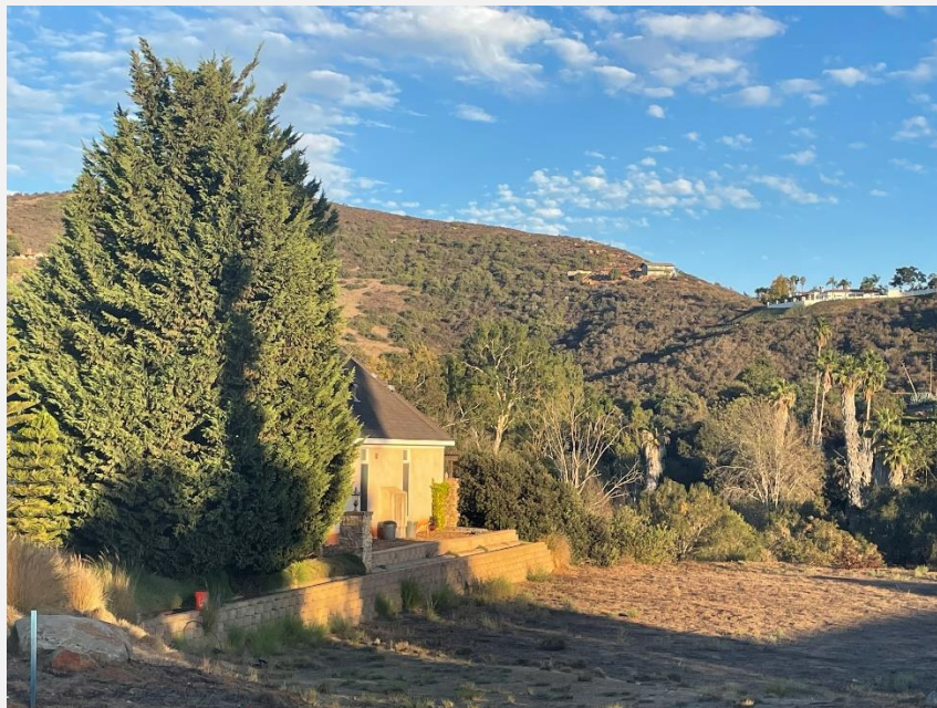
Photograph 12: Photograph taken from Vista Grande Drive looking southeast. The pictured home is at higher risk for structural ignition to due an absence of defensible space and flammable plant species directly adjacent to the home.
