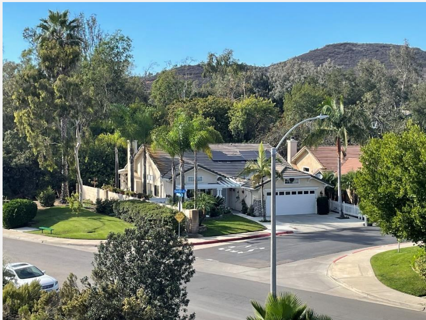
Photograph 2: Photograph taken near the intersection of Green Oak Road and Sycamore Avenue looking west across a community designated within the Wildland Urban Interface. Dense vegetation with high fuel continuity adjacent to this home increases the likelihood of structural ignition during a wildfire and limits the capacity for successful structure protection.
