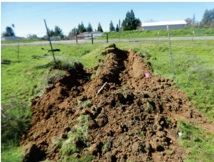
Photo #33: Western soil piles Trench T-9 - No significant staining or odor
