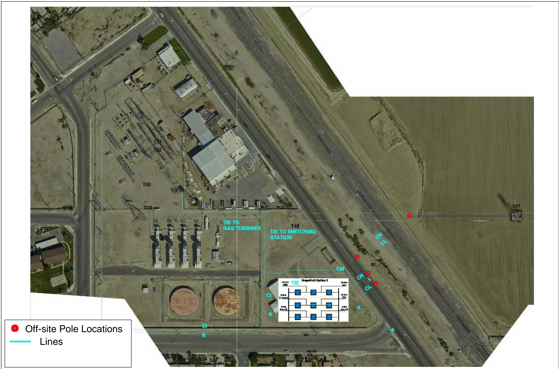
Figure 3 Grapefruit Switching Station Site Plan
