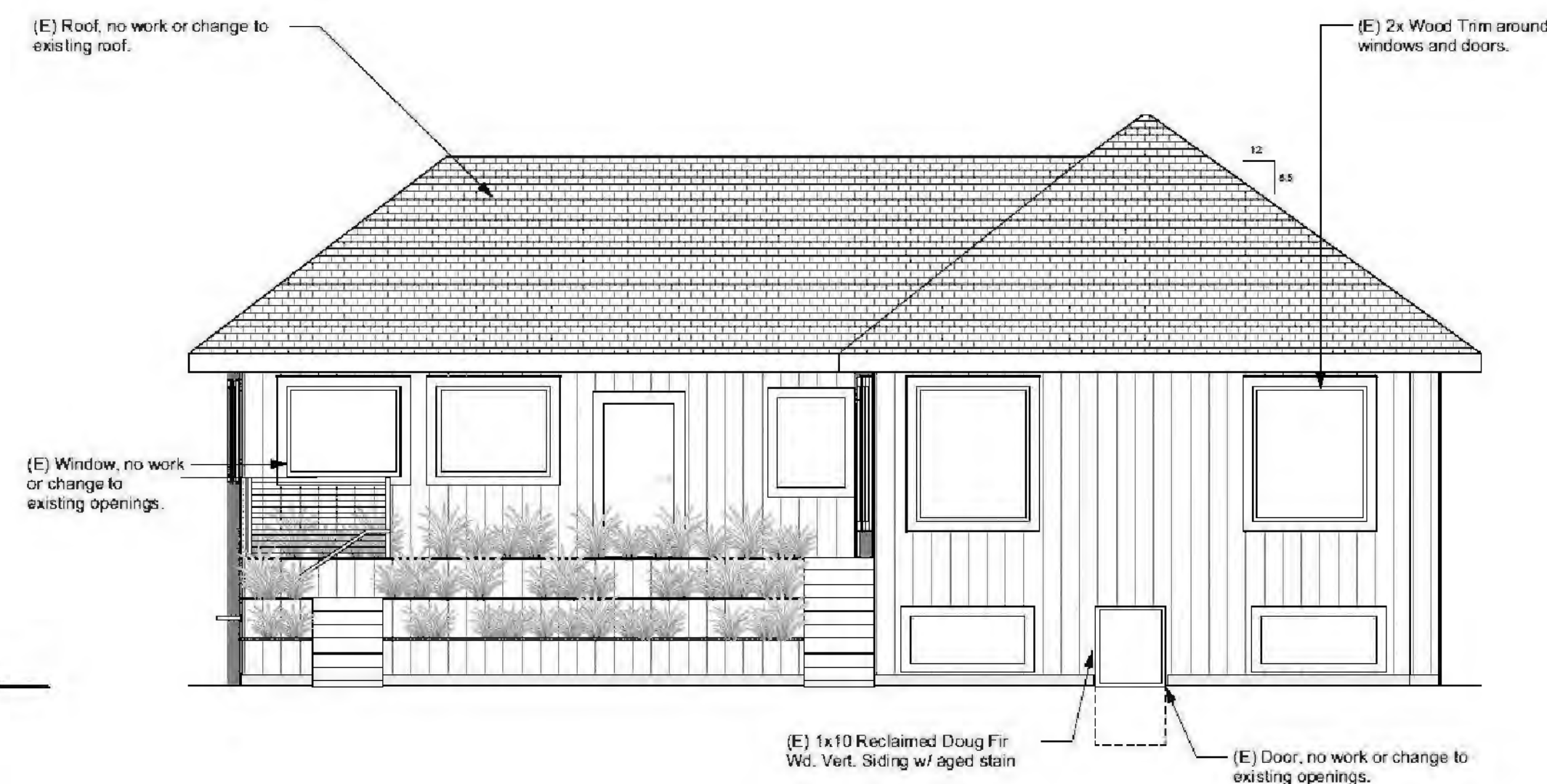
1 Existing North Elevation: House Scale: 3/16" = 1'-0"
