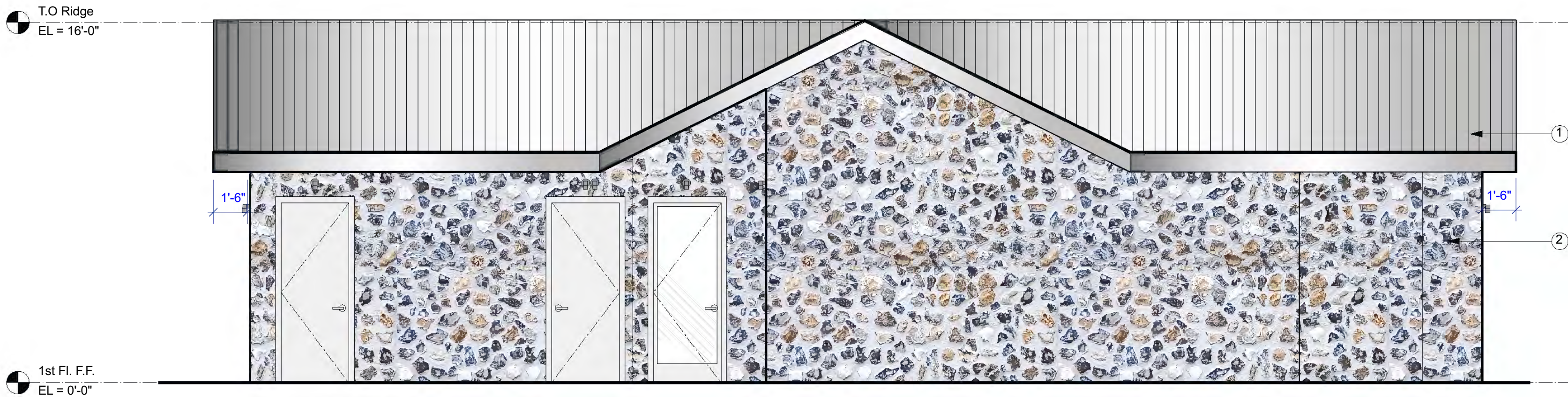
4 Proposed West Elevation Scale: 1/4" = 1'-0"
