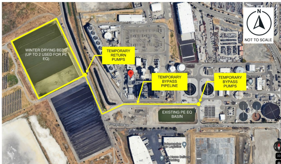
Figure 3-5 Temporary Pipeline and Winter Bed Use During Construction
