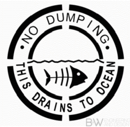
CATCH BASIN STENCILING DETAIL NTS
