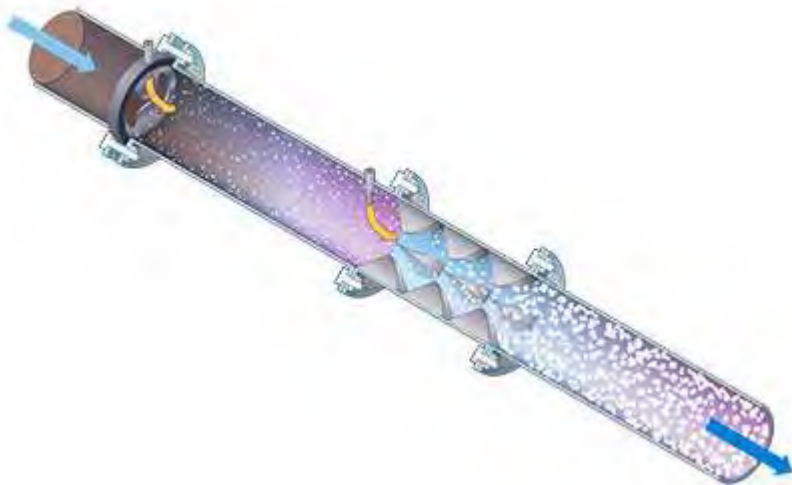
Figure 4: Coagulation/Flocculation Static Mixer (Westfall Mfg)
