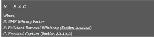
The pollutant removal efficiency (E) was determined based upon the TAPE documentation provided by BioClean to support the Kraken curb inlet filter unit. Per this TAPE, the Kraken's average reduction of Phosphorus (TP) was rated at 72%. Given that TP is a pollutant of concern as discussed previously within the WQMP, the removal rate of 0.72 for TP was used as the treatment efficiency of the BMP.
