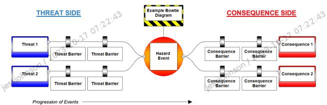
Figure 3-1 - Example Bowtie Diagram
