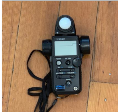
Figure 5: Light meter used for luminance and illuminance measurements
