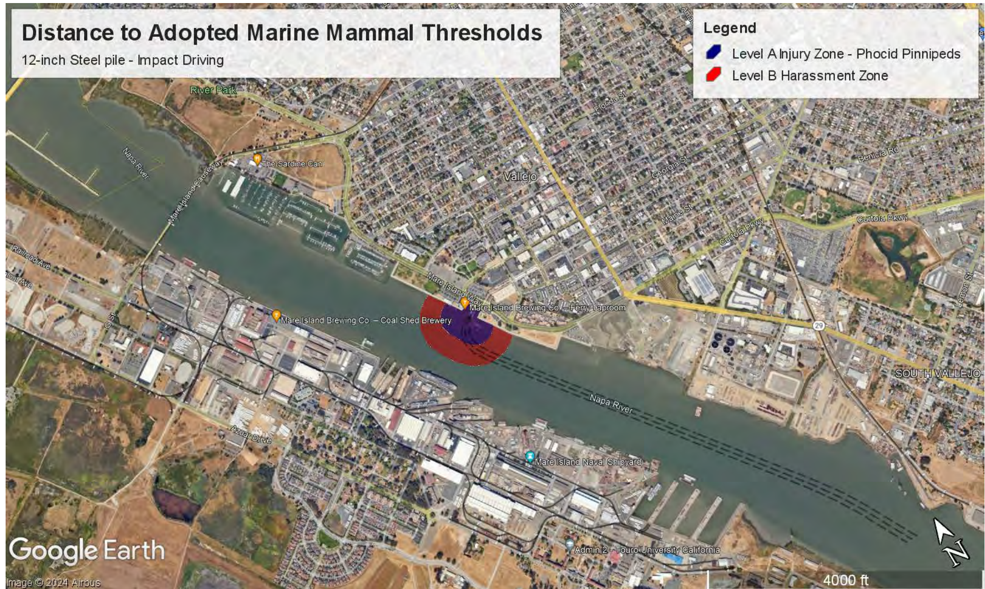
FIGURE A3 Distance to Marine Mammal Thresholds for 12-inch steel piles impact driven (Google Earth 2024)
