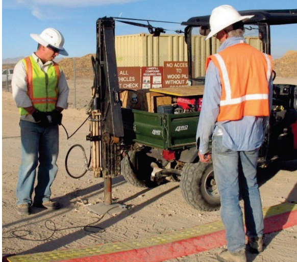
Figure 2-3. ATV-Mounted Geophysical Hammer Specified for Use for the Proposed Design Level Geotechnical Investigations
