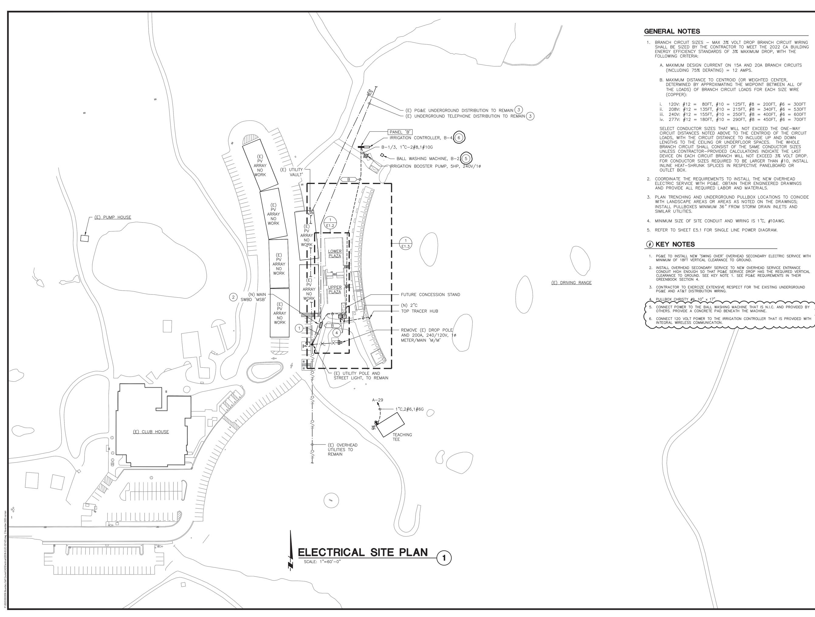
1. BRANCH CIRCUIT SIZES - MAX 3% VOLT DROP BRANCH CIRCUIT WIRING SHALL BE SIZED BY THE CONTRACTOR TO MEET THE 2022 CA BUILDING ENERGY EFFICIENCY STANDARDS OF 3% MAXIMUM DROP, WITH THE
