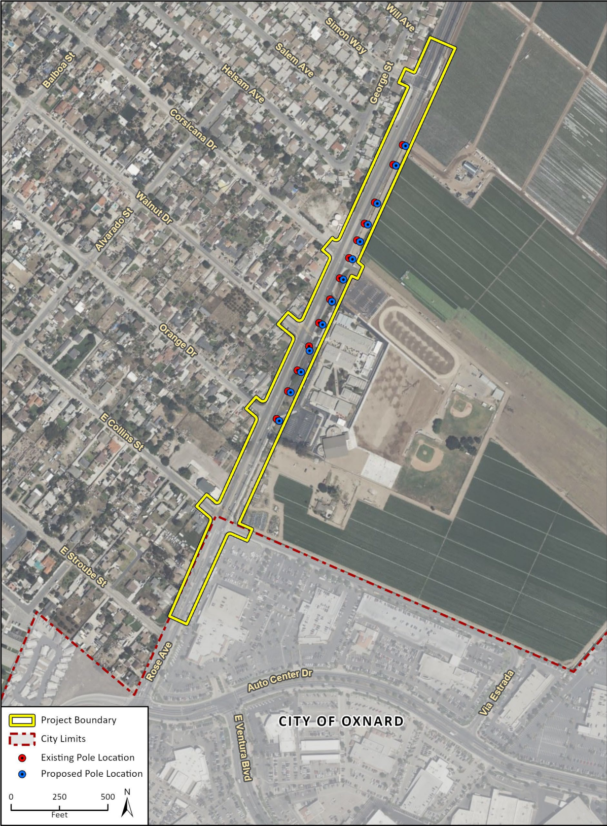
Figure 5 Proposed Utility Pole Relocations – Southern Segment
