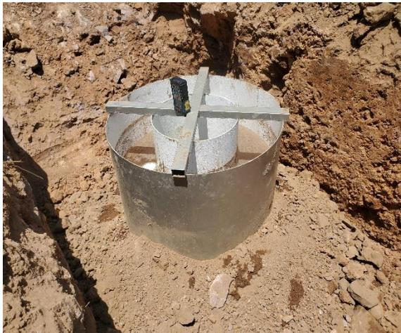
Figure 22: Position of laser meter and method of reading level of the water.
