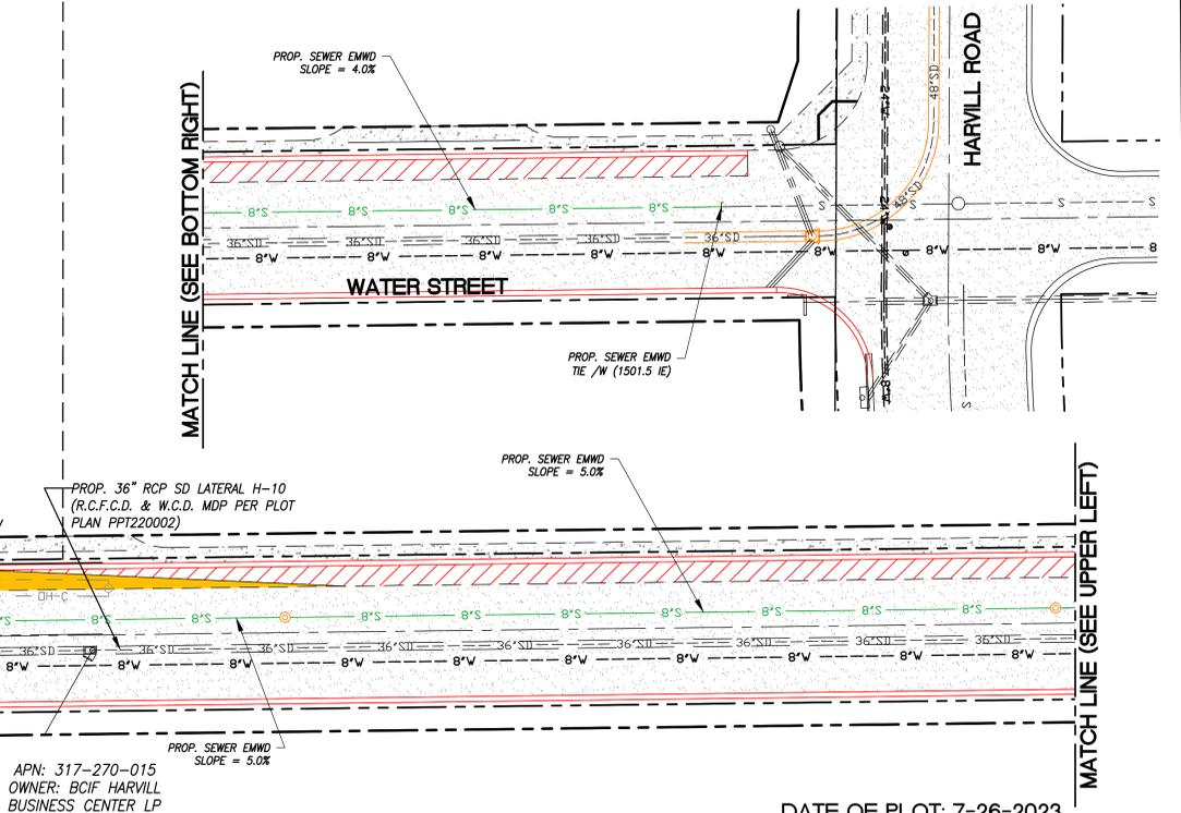
PROPOSED 36" STORM DRAIN (L=665± L.F.) R.C.D.F.C. & W.C.D. LATERAL H-10 MDP (SD)
