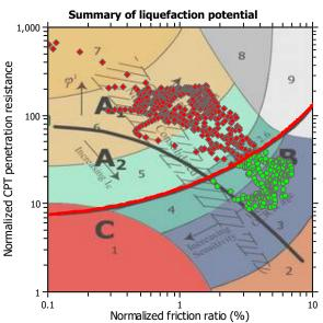
Zone  $A_1$ : Cyclic liquefaction likely depending on size and duration of cyclic loading Zone  $A_2$ : Cyclic liquefaction and strength loss likely depending on loading and ground
