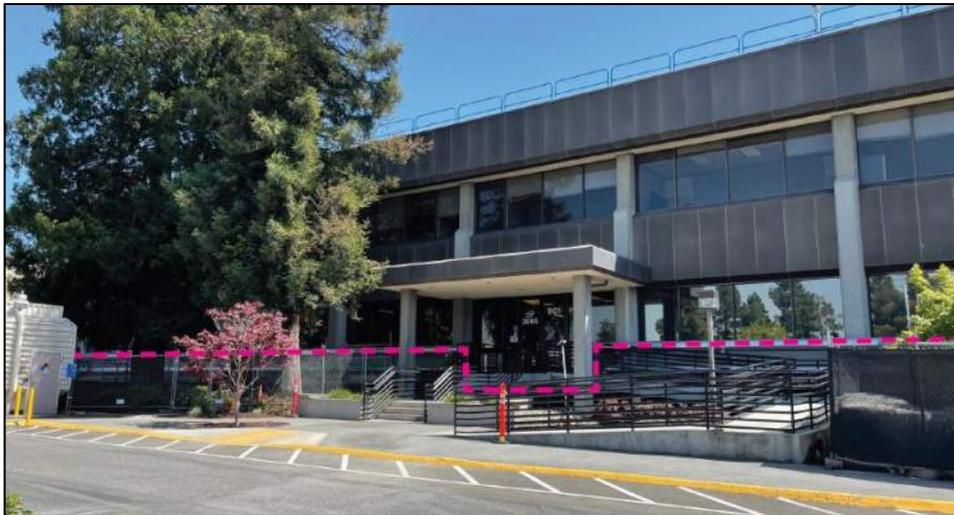
Figure 61. Illustration depicting the location of the proposed location of the recycled water pipeline along the north façade of SC1 (dashed pink line), aligned with the current location of an existing pipeline. The new pipeline would be routed underneath the landing platform at the main entrance, at center.
