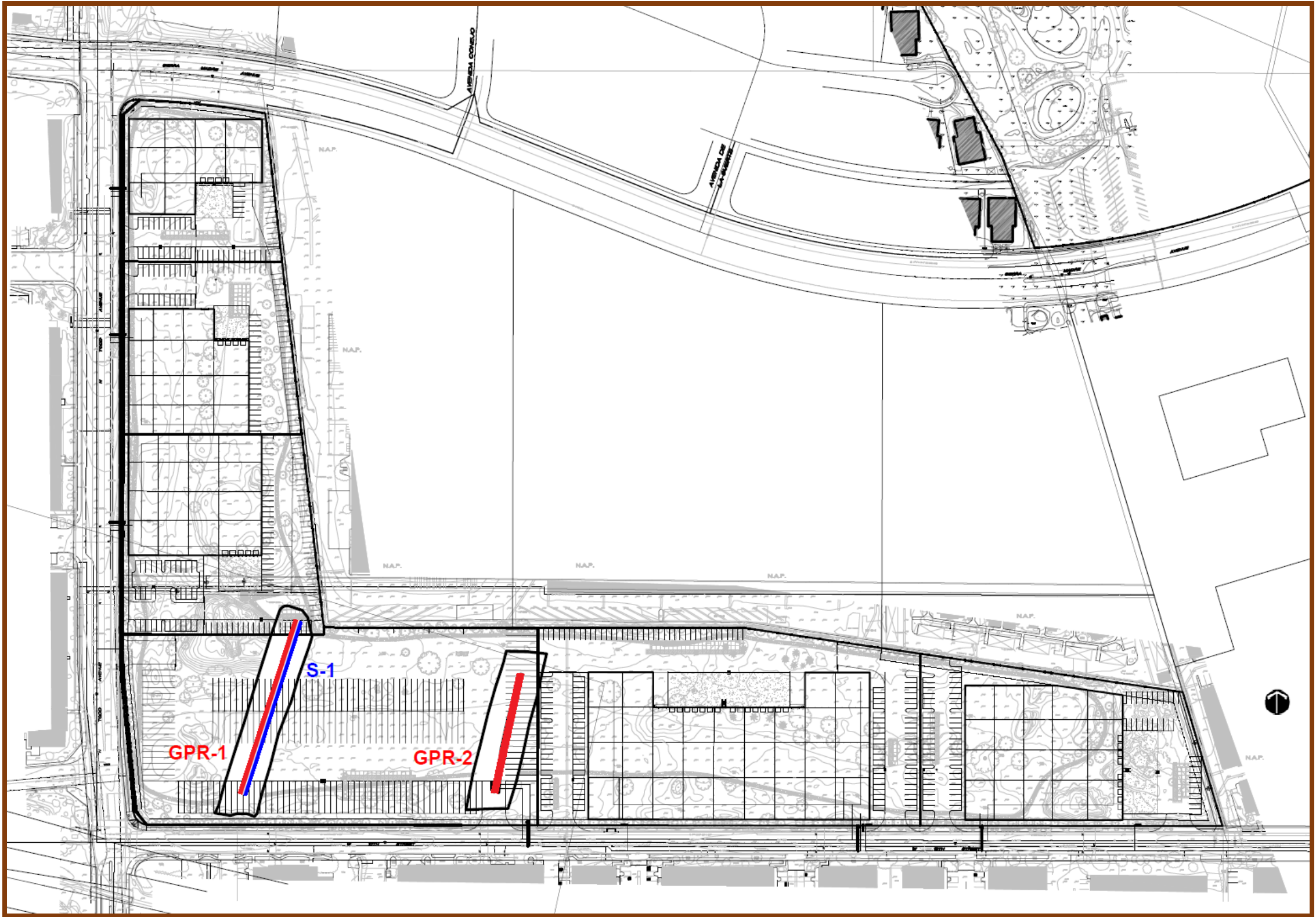
Base Map: Provided by client; Seismic survey line (S-1) shown as blue line, GPR survey lines GPR-1 & GPR-2 shown as red lines.
