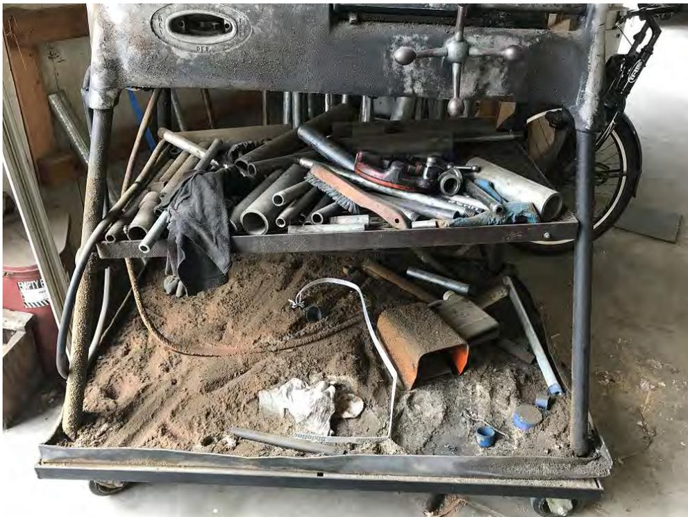
Pipe threading machine in the Mill Works shop.
