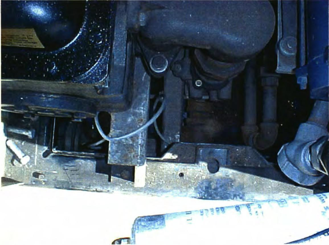
This is the south dispenser (#2). The sensor was not properly placed here either. Some liquid can be seen to right.
