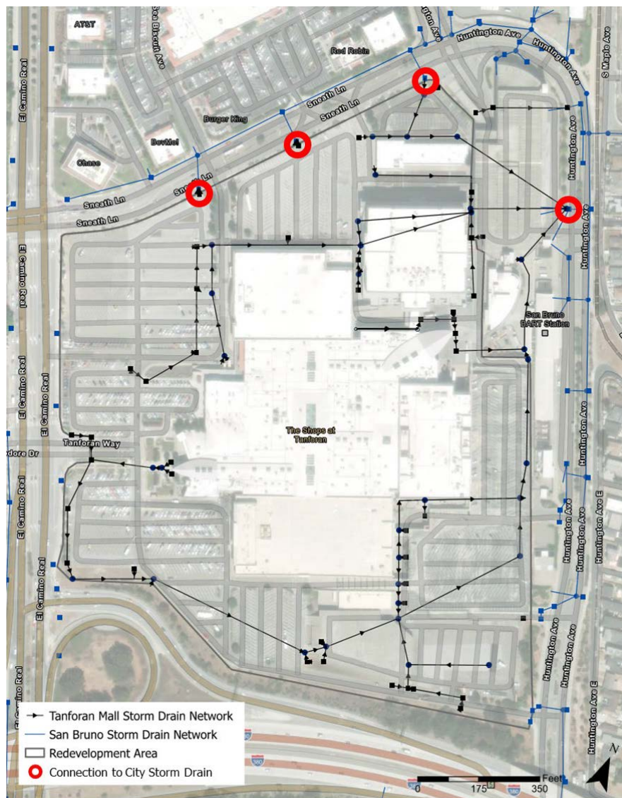
Figure 1. Existing Storm Drain on Tanforan Mall with Multiple Outlets
