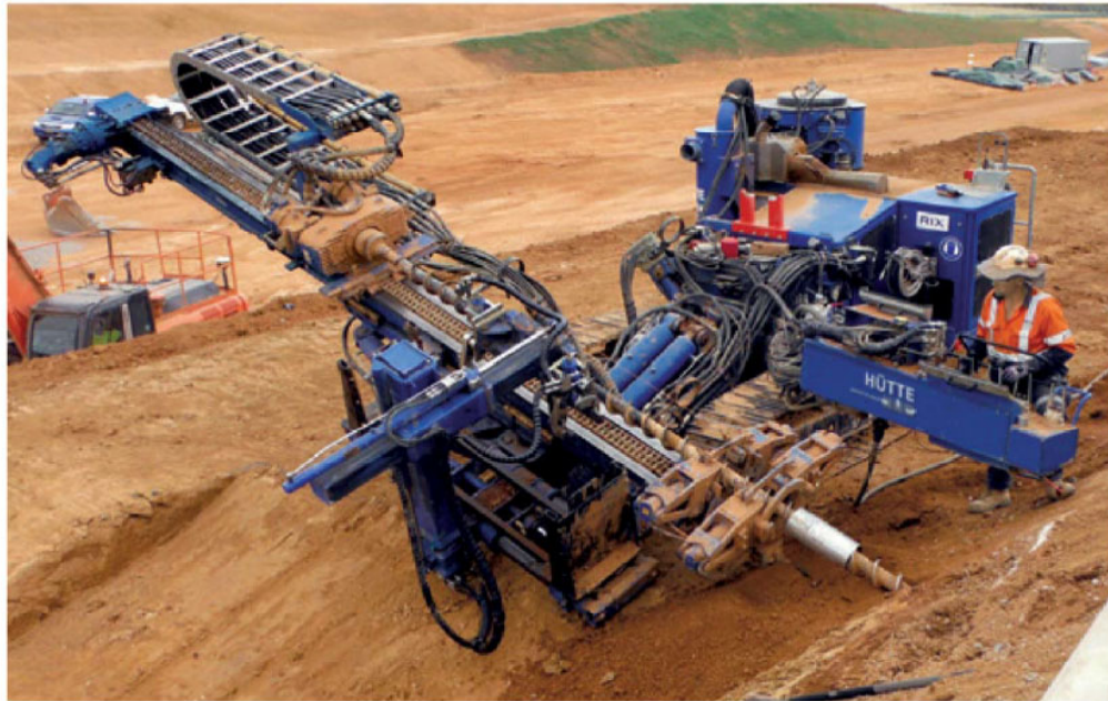
Image 34 – Example Ground Anchor Drill Rig (Hütte HBR 605-4)
