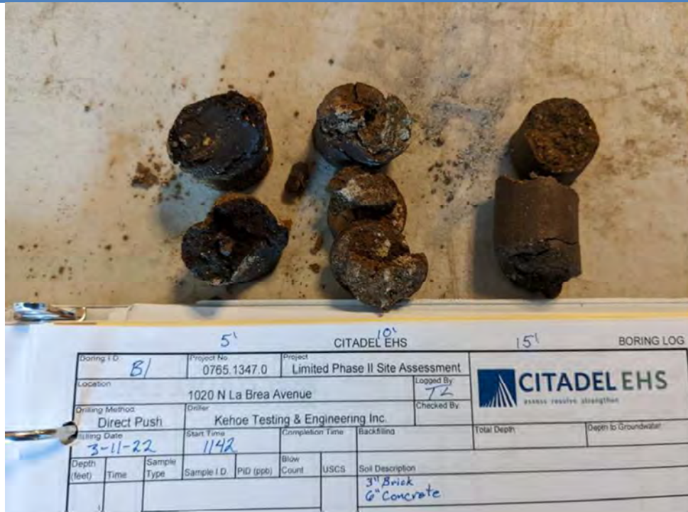
PHOTO 5: Split samples from Boring B1 (3/11/22).
