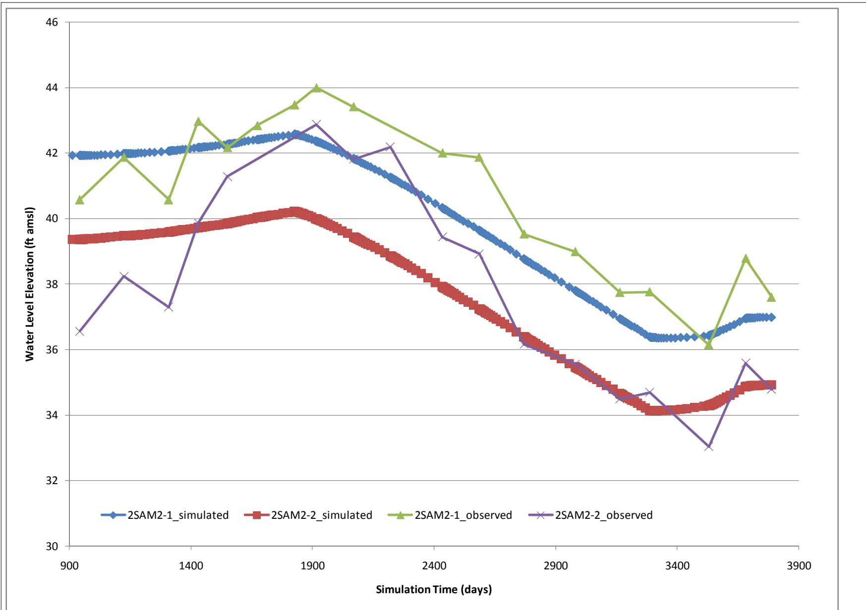
Figure 5.29. Hydrographs of Simulated and Observed Water Level Elevations, 2SAM2-1 and 2SAM2-2
