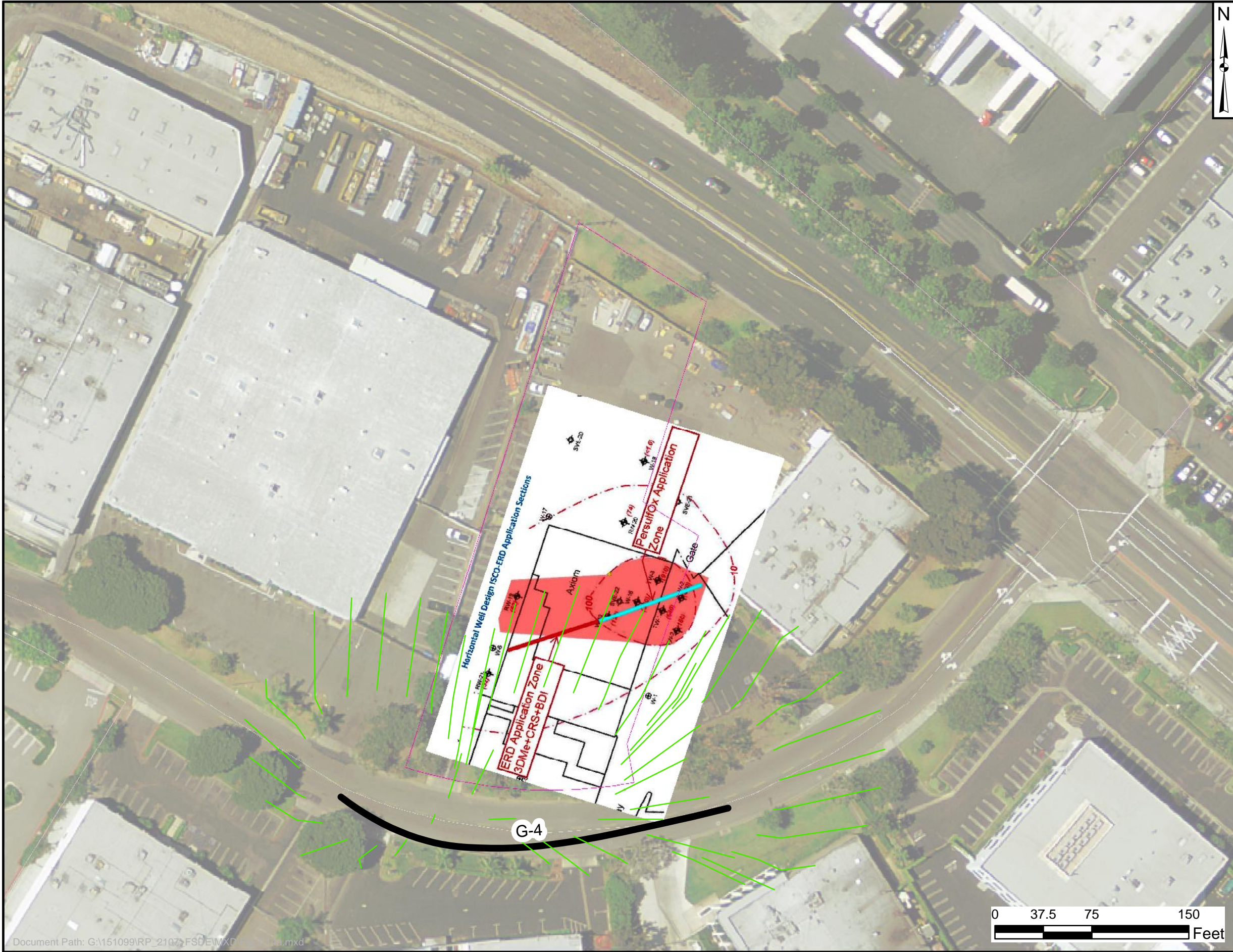
FIGURE 7-14A TROY COMPUTER PROPOSED HORIZONTAL WELL DESIGN ISCO-ERD APPLICATION SECTIONS AND OCWD MODEL SIMULATED GROUNDWATER PARTICLE TRACKS ORANGE COUNTY WATER DISTRICT SOUTH BASIN
