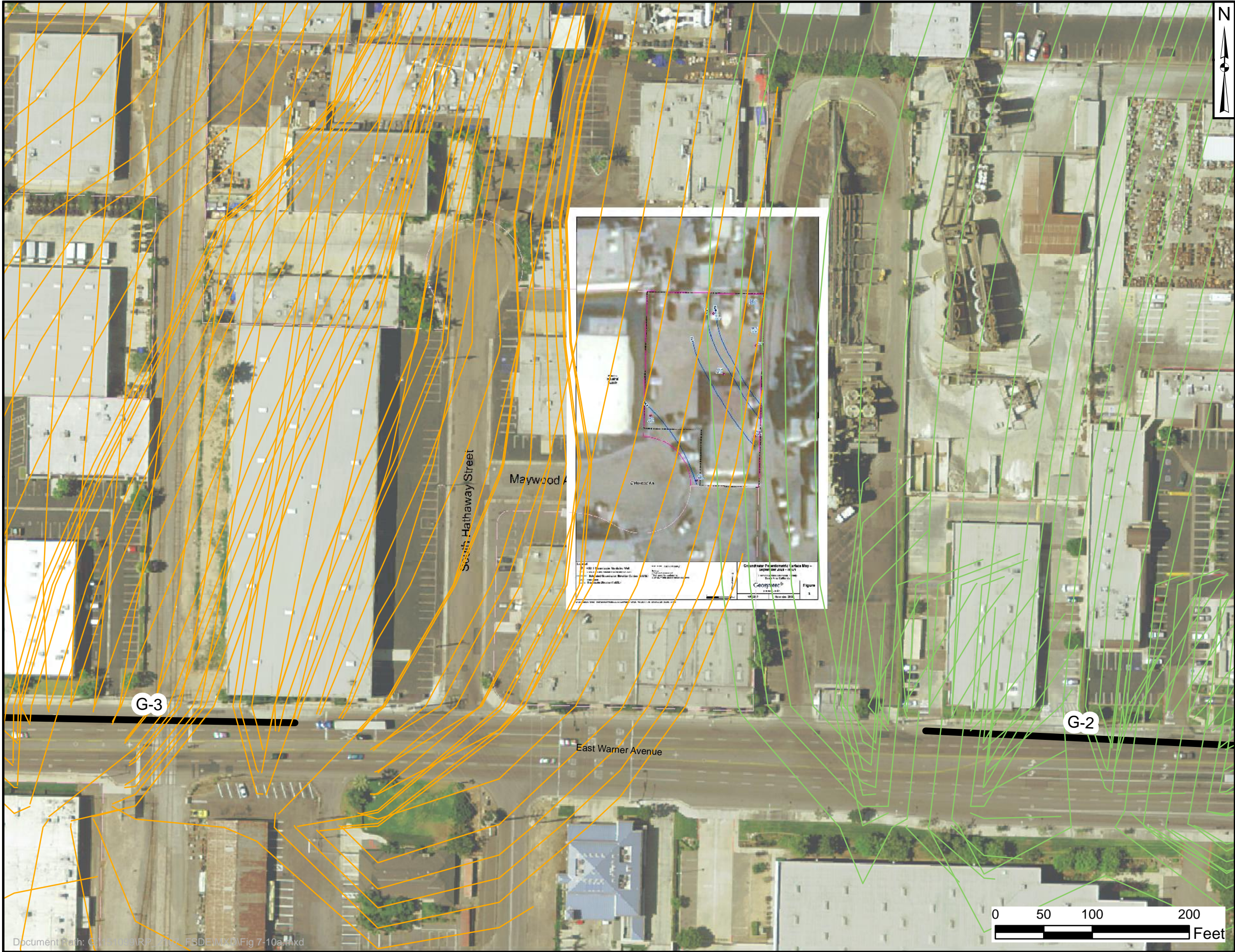
FIGURE 7-10A COMPARISON OF OCWD MODEL SIMULATED GROUNDWATER PARTICLE TRACKS VERSUS PUBLISHED HSU 1 GROUNDWATER ELEVATION CONTOURS, SOCO WEST, INC., FORMER SERVICES CHEMICAL ORANGE COUNTY WATER DISTRICT SOUTH BASIN
