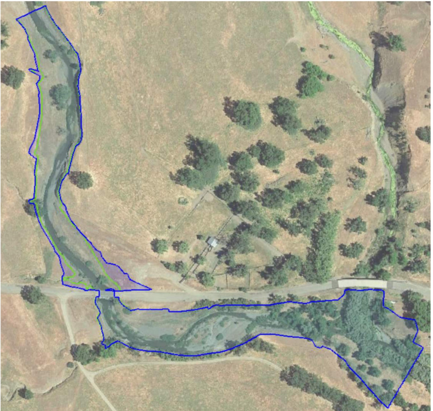
Figure 4. Water surface extents comparison between existing (blue) and proposed (green) conditions for the 100-yr discharge.
