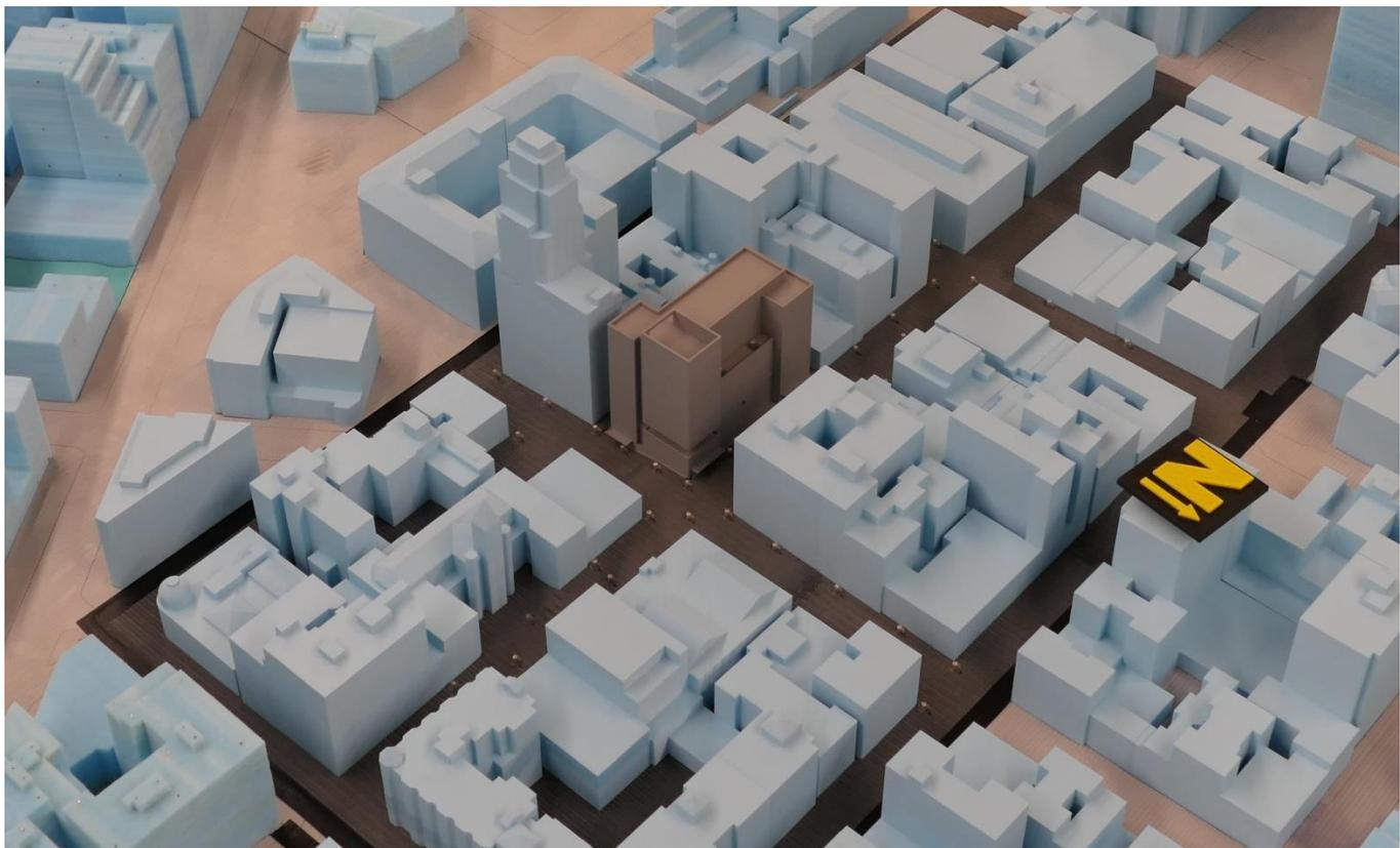
*Image 2D: Photographs of Wind Tunnel Test Model – Existing + Project (Academic Heavy) Configuration*
