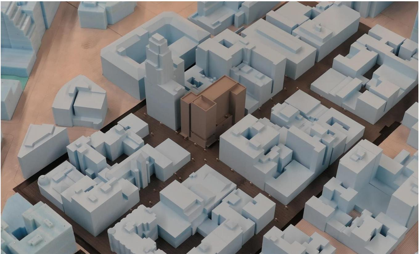
*Image 2B: Photographs of Wind Tunnel Test Model – Existing + Project (Academic Light) Configuration*
