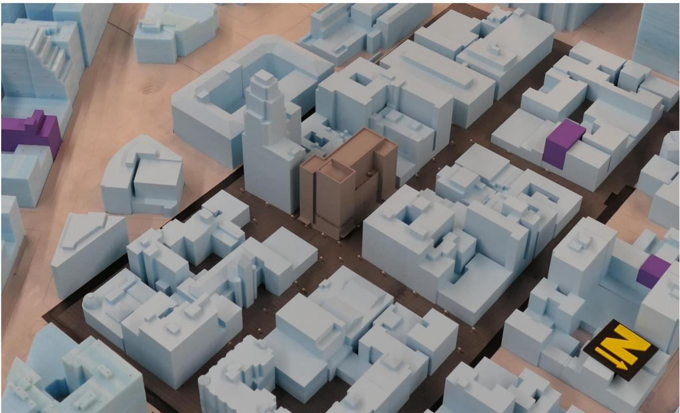
Image 2E: Photographs of Wind Tunnel Test Model – Project + Cumulative (Academic Heavy) Configuration
