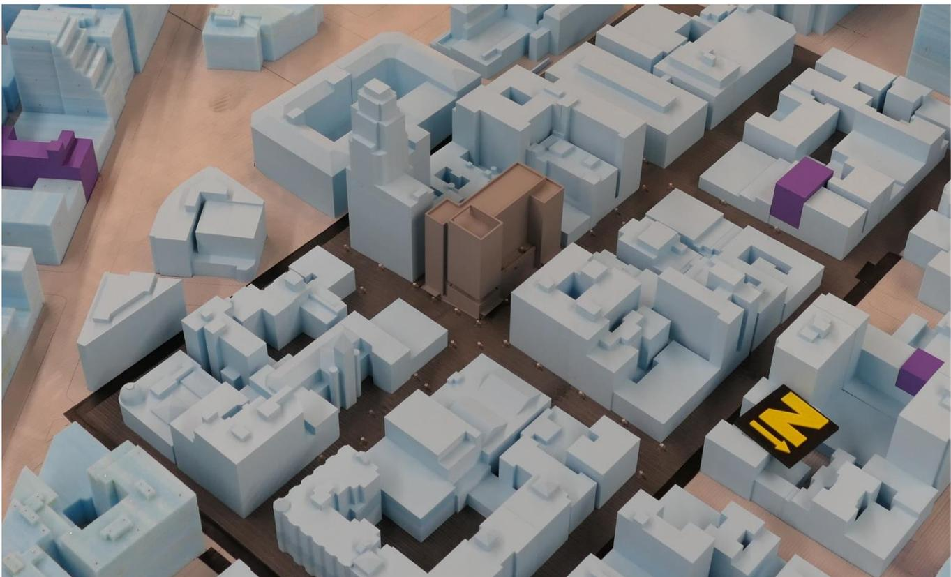
*Image 2C: Photographs of Wind Tunnel Test Model – Project + Cumulative (Academic Light) Configuration*
