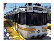
**Metro Rail:** Metro operates heavy rail (HRT) and light rail (LRT) transit lines in underground tunnels, along streets, off-street in dedicated ROW, and above street level on elevated structures. Heavy rail trains are powered by a "third rail" along the tracks. Light rail vehicles are powered by overhead catenary systems (OCS). To support rail operations, Metro owns and maintains traction power substations (TPSS), maintenance yards, and other infrastructure.
