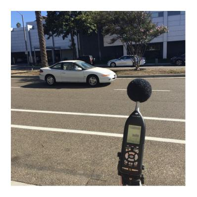
Summary File Name on Meter LxT\_Data.008 SLM 0005425 LxT Data 008.00.ldbin File Name on PC Serial Number 0005425 SoundTrack LxT® Model **Firmware Version** 2.301 User JC Location Redondo Beach **Job Description** CORB-01 Redondo Beach GP Note Measurement Description Start 2018-09-12 17:37:58 Stop 2018-09-12 17:52:59 Duration 00:15:01.3 **Run Time** 00:15:01.3 **Pause** 00:00:00.0 **Pre Calibration** 2018-09-12 10:29:15 **Post Calibration** None **Calibration Deviation**
