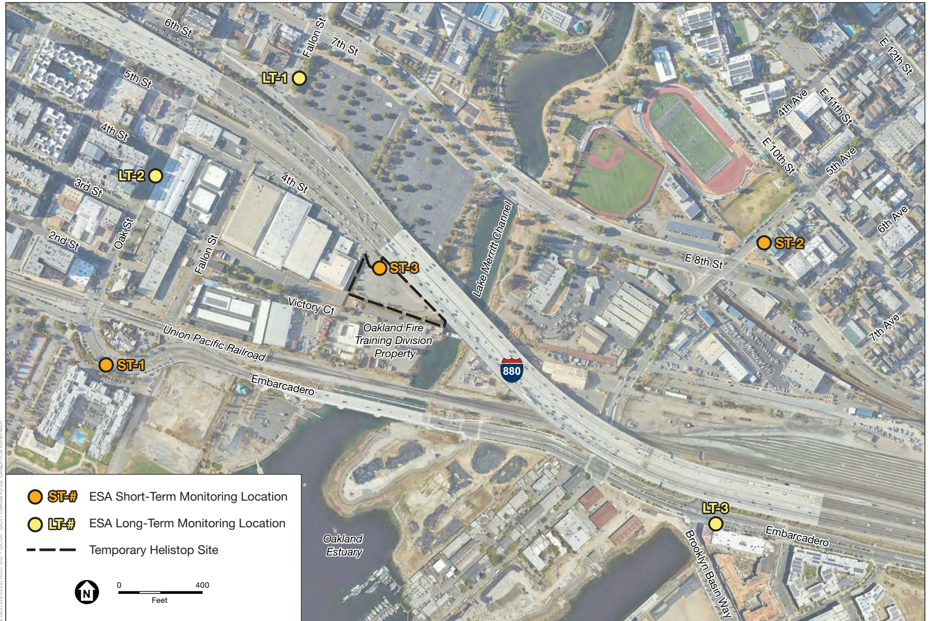
Figure 8.3-14 Noise Monitoring Locations in the Peralta Site Temporary Helistop Vicinity
