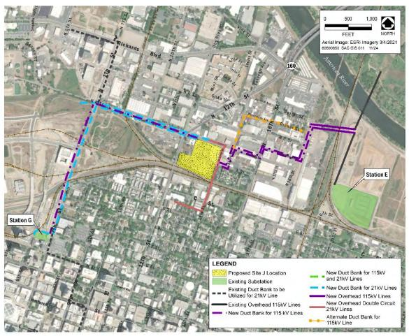
Figure 6-2: Alternative C Transmission Line Routing Option
