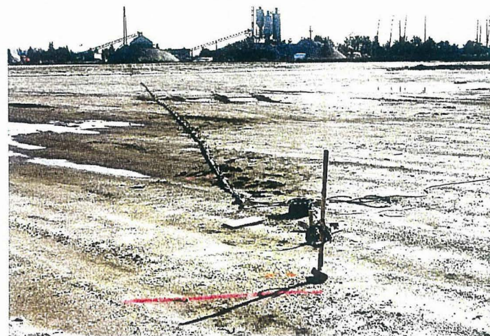
LANDSTREAMER USED FOR MASW SURVEY
