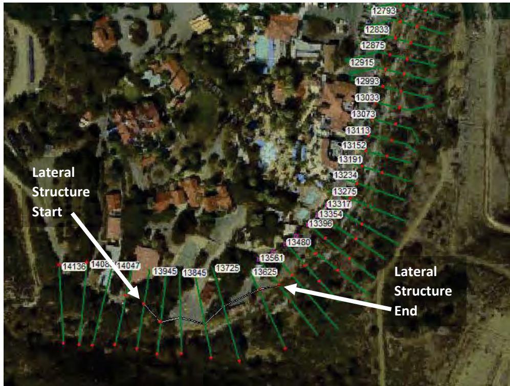
Figure 23. HEC-RAS Lateral Structure Location
