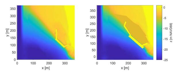
Figure 3-10: Topo-bathymetry of the existing pier and breakwater layout (left panel) and proposed facility layout (right panel) in the computational domain. Note: The computation domain for the proposed facility extends slightly below the origin (0,0).
