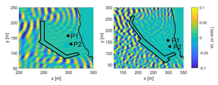
Figure 3-11: A snapshot of waves diffracting around the existing pier (left panel) and proposed pier (right panel) at t= 500 seconds. Two points of interest (P1 and P2; black circles) are labelled to indicate where further analysis is conducted. Note: The axis extents are not equivalent between panels.
