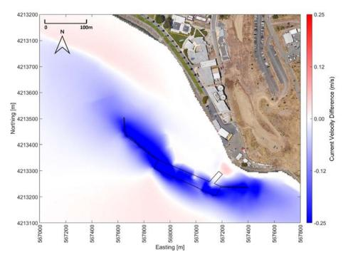
Figure 3-23: Current velocity difference during Flood Tide - Proposed Pier Design vs. Existing Pier. Blue areas indicate reduced current speed and red areas show increased speed for the proposed pier.
