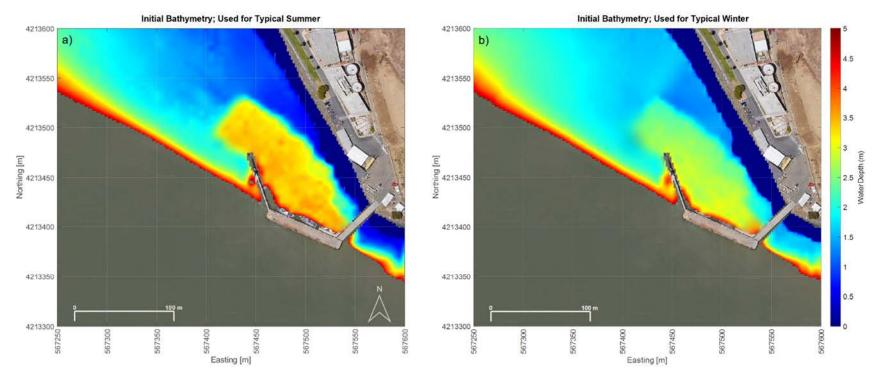
Figure 3-31: Existing pier with 2019 post-dredge bathymetry used for summer simulation 1 (left) and with updated end-of-summer bathymetry for the winter simulation 2 (right)
