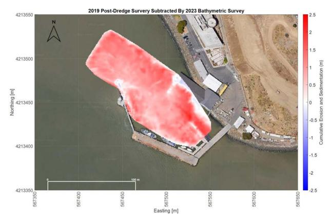
Figure 3-30: Difference between the 2019 post-dredge and 2023 seabed elevation. Red and blue areas show sediment build-up and erosion, respectively.
