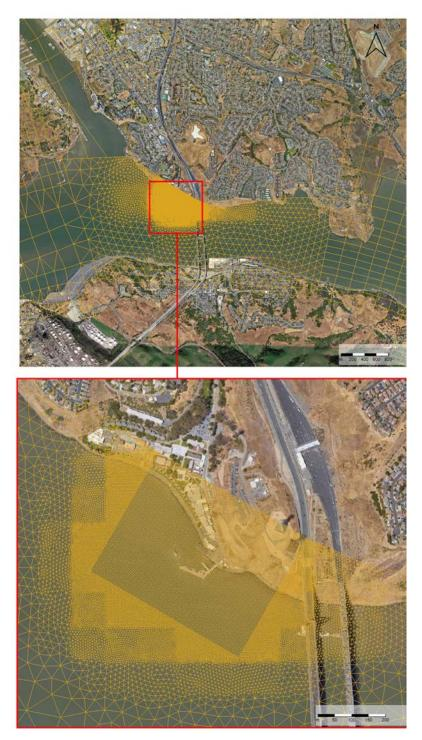
Figure 3-16: Model domain at project site; Cell size ranging from 20 m to 4 m
