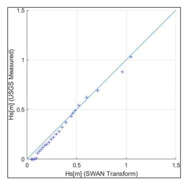
Figure 3-4: Q-Q plot comparison of measured and modelled significant wave heights (Hs) in San Pablo Bay at USGS\_PCT location
