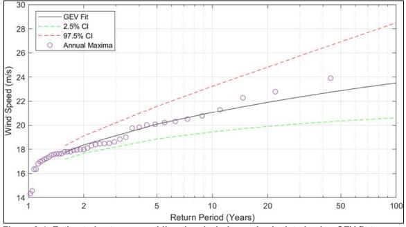
Figure 2-4: Estimated extreme omnidirectional wind speed calculated using GEV fit to annual maxima of hindcast wind
