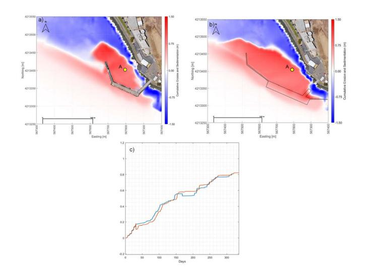
Figure 3-33: (a) Morphological change after 1 year (typical summer followed by typical winter, with MORFAC 6) for the existing pier (b) Morphological change after 1 year (typical summer followed by typical winter, with MORFAC 6) for the proposed pier (c) Timeseries of sedimentation for existing and proposed pier configurations at point A (yellow circle).
