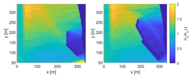
Figure 3-13: Wave height ratios between significant wave height ( $H_s$ ) and offshore significant wave height ( $H_o$ ) across the SWASH domain for the (left panel) existing and (right panel) proposed pier layouts. The top and bottom of the domain are not shown as they serve as dissipative sponge layers.
