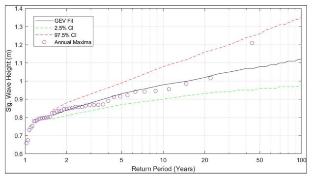
Figure 3-9: Estimated extreme significant wave height at the site using GEV distribution fit to annual maxima
