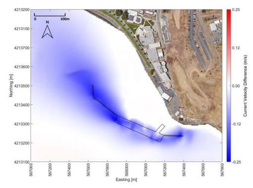
Figure 3-24: Current velocity difference during Ebb Tide - Proposed Pier Design vs. Existing Pier. Blue areas indicate reduced current speed and red areas show increased speed for the proposed pier.
