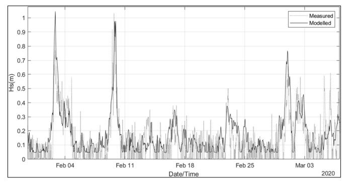
Figure 3-5: Time series comparison of 3 large wave events (measurements vs. SWAN model prediction) in 2020
