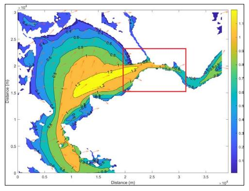
Figure 3-1: Contours of significant wave height (m) in the Primary Domain predicted by the SWAN wave model for a 20 m/s WSW wind (Secondary Domain: red box)
