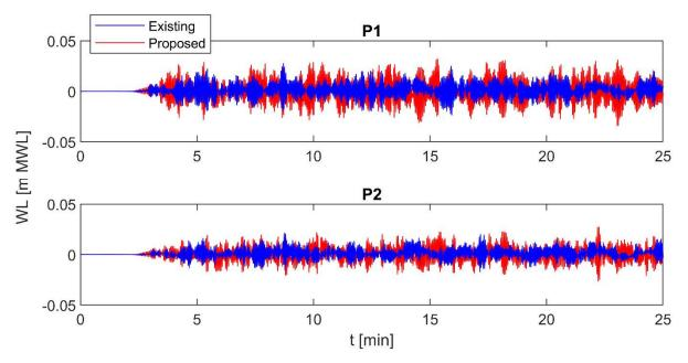
Figure 3-12: Water level time series at P1 (top; refer to Figure 3-11 for location) and P2 (bottom; refer to Figure 3-11 for location) for the existing (blue) and proposed (red) pier layouts
