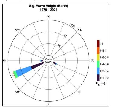
Figure 3-6: Wave rose of hindcast significant wave height at the site
