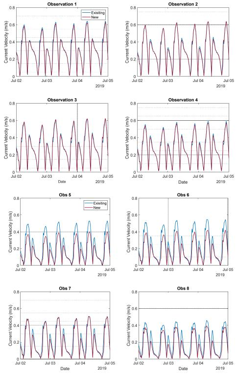
Figure 3-26: Comparison of Currents at Locations 1-8 for Existing and Proposed Pier Designs
