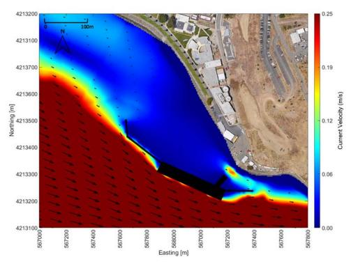
Figure 3-21: Current Velocity during Peak Flood Tide with Proposed Pier; July 03, 2019, at 06:00 UTC
