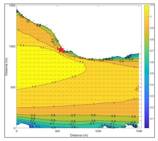
Figure 3-3: Contours of significant wave height (m) in the Tertiary Domain predicted by the SWAN wave model for a 20 m/s WSW wind (Site: red star)
