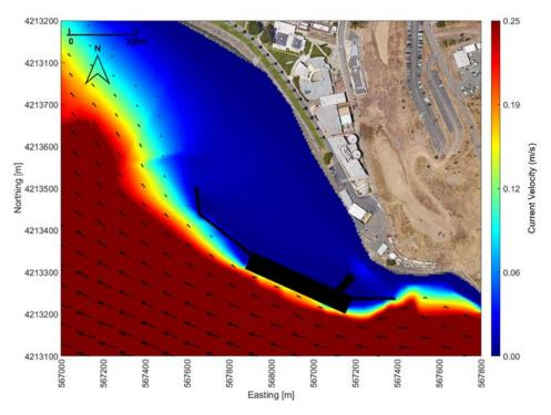
Figure 3-22: Current Velocity during Peak Ebb Tide with Proposed Pier; July 03, 2019, at 11:00 UTC
