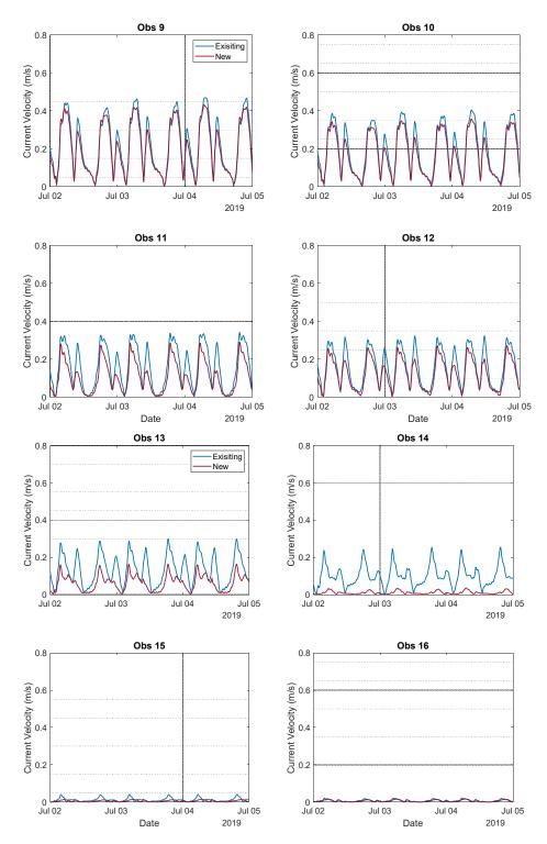
Figure 3-27: Comparison of Current Speed at Locations 9-16 for Existing and Proposed Pier Designs
