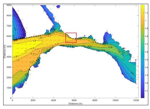
Figure 3-2: Contours of significant wave height (m) in the Secondary Domain predicted by the SWAN wave model for a 20 m/s WSW wind (Tertiary Domain: red box)
