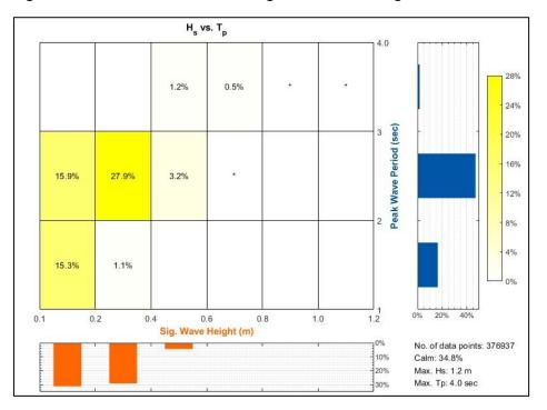
Figure 3-7: Bivariate distribution of hindcast significant wave height and peak wave period at the site
