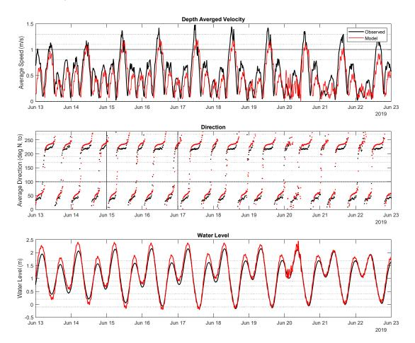
Figure 3-18: Comparison of Current Velocity and Water Level – Numerical model vs. USGS ADCP Data
