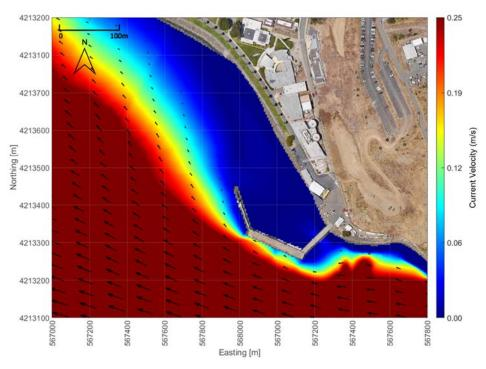
Figure 3-20: Current Velocity during Peak Ebb Tide with Existing Pier; July 03, 2019, at 11:00 UTC
