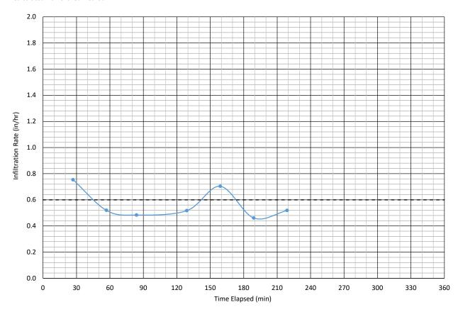
Project: <u>Hesperia 29-Acre Business</u> Project No.: 2202-09 Date: 3/4/2022 Test Hole No.: P-3 Tested By: Water Temp.: USCS: Depth of Test Hole: 48 inches Air Temp.:
