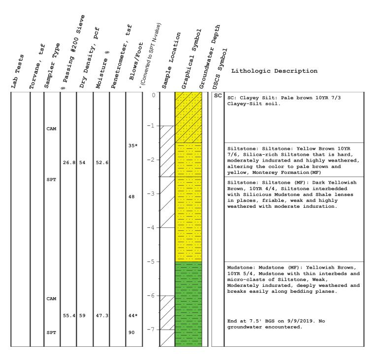
\*Sampling was performed by Denovo Drilling using a hydraulic portable drill rig equipped with solid flight augers.
