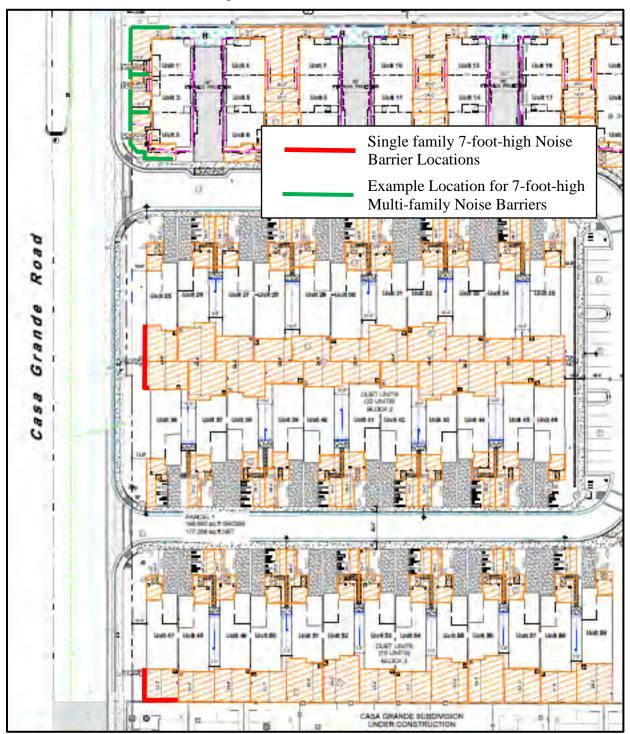
Figure 2: Site Plan with Noise Barrier Locations
