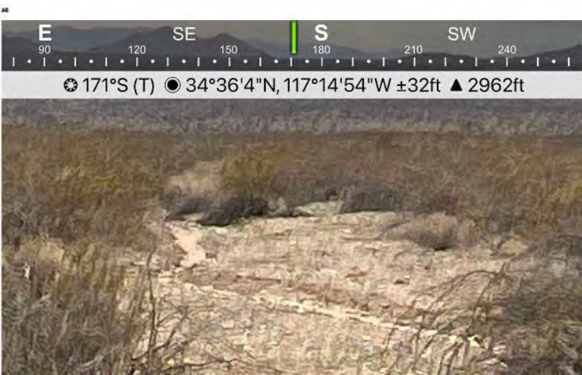
Photograph # 6. Rilling and ponding - no change in vegetation, cobble or other ordinary high water mark indicators. Appears to be an off-highway vehicle tracks. Signature ended in the middle of the Project Site.
