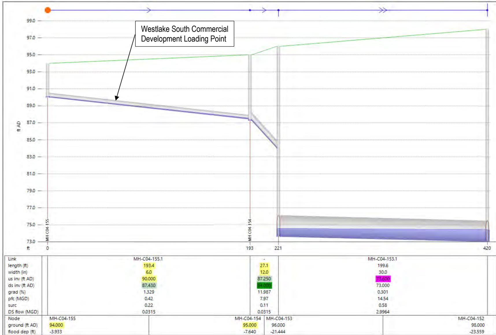
Figure 4: Model Profile of Lake Merced Boulevard Sewer MH-C05-171 to MH-C04-105
