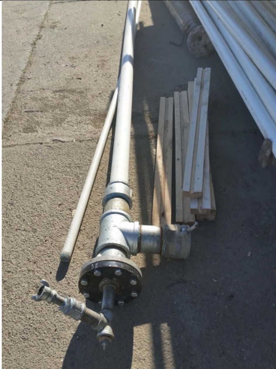
Head assembly for dual swab development tool.
