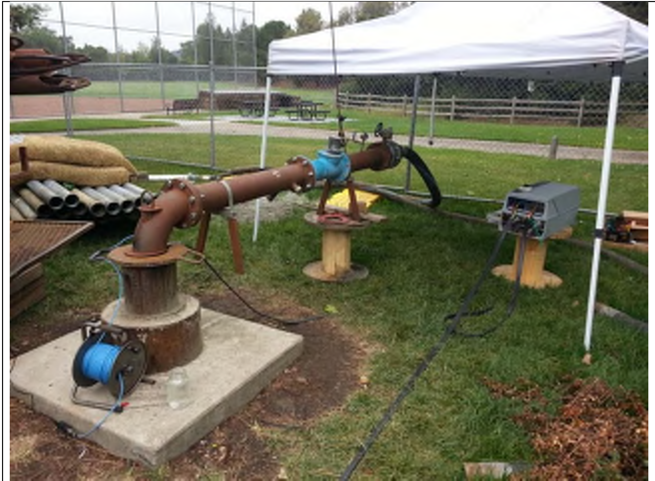
Configuration of well head during pumping tests.
