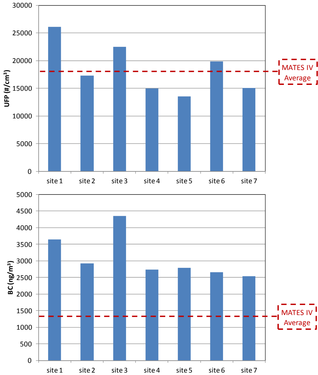
Figure 5-13 - Average UFP and BC levels measured at the seven temporary sites surrounding San Bernardino Railyard.
