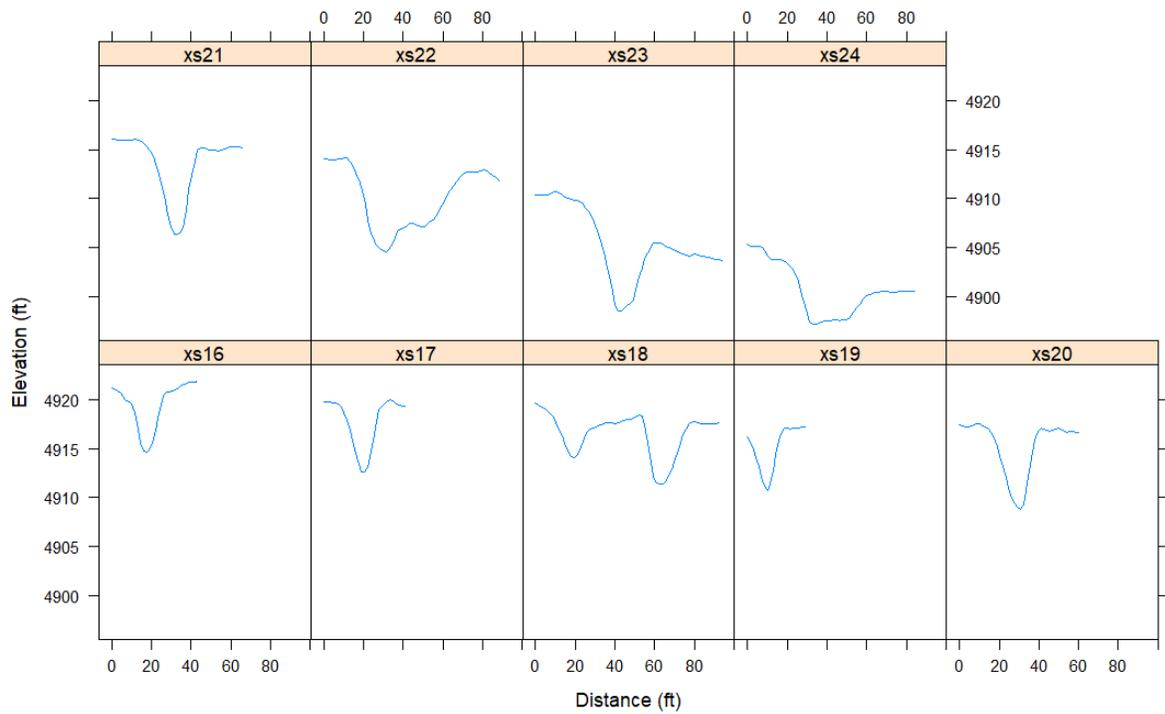
**Figure B9. Cross sections plots for channel fill 10 (CF10) in Area 4, Finger Fen, as shown in Figure 5. River left is on the left of the plot. River right is on the right of the plot. Bottom left panel is furthest upstream.**
