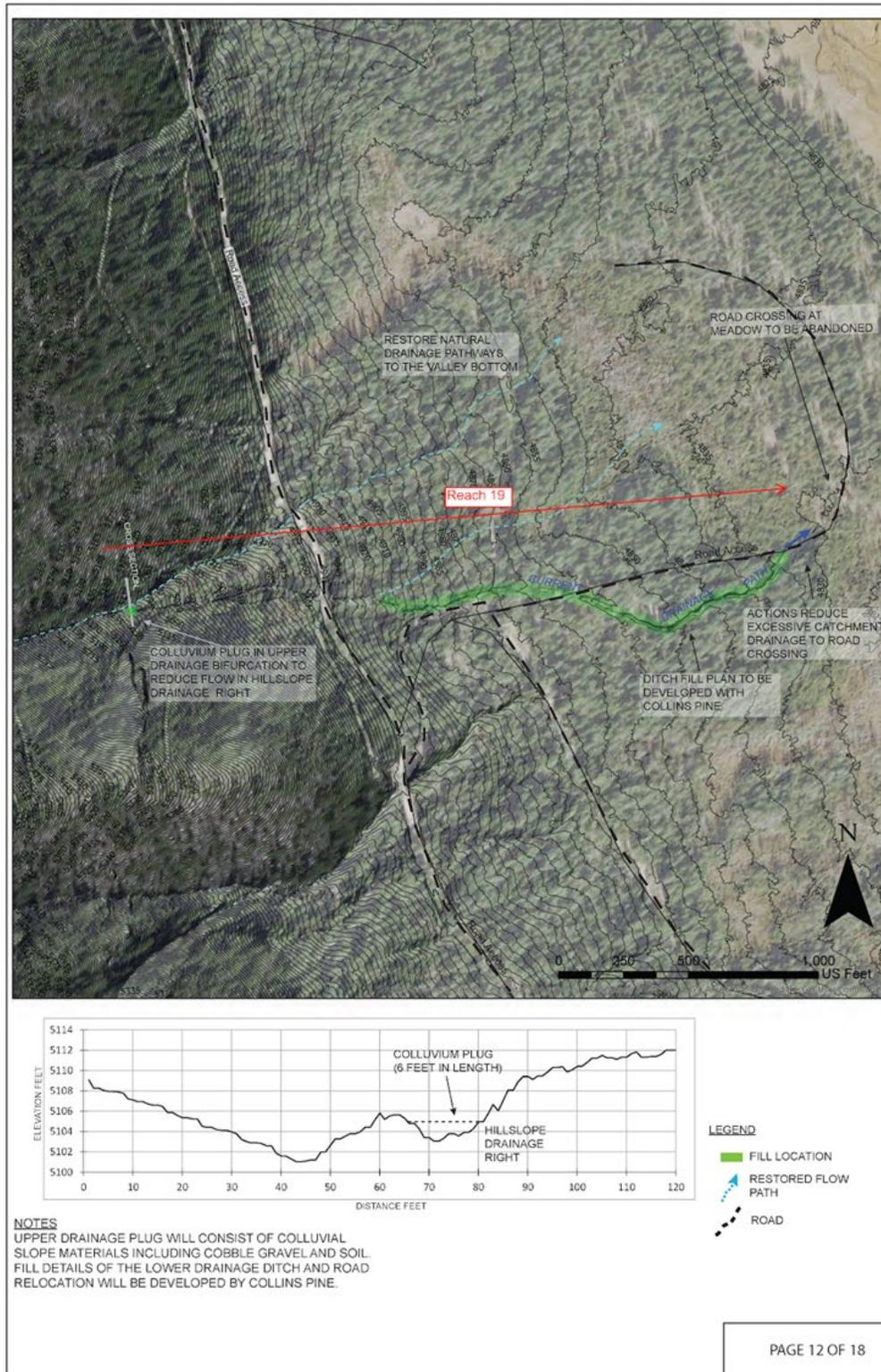
**Figure 22: Design Plan View and Cross Section for Area 19**
