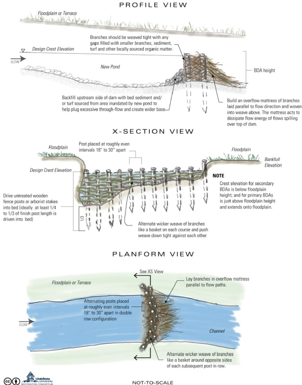
**Figure A1. Typical schematic sketches of a modified post-line wicker weave BDA with a double row of alternating posts, a convex crest orientation, and an overflow mattress to dissipate flow over the top of the dam (Wheaton et al. 2019)**
